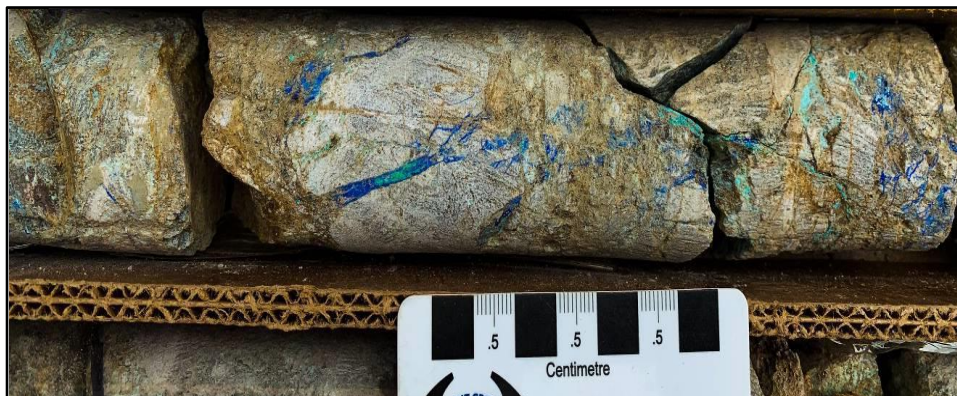
Malachite, azurite and chrysocolla in fractured Pinal Schist DDH M-3, 294.5m
