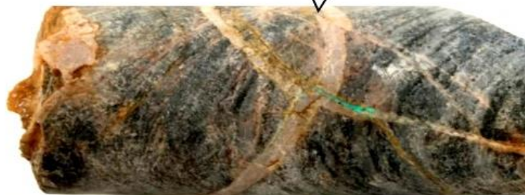
Malachite in quartz vein Pinal Schist, 354.3m
