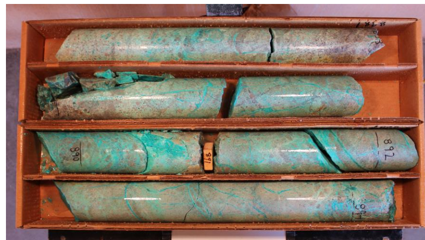
Malachite and chrysocolla in Pinal Schist, DDH VD14-06 (886.0 – 894.3ft) 3.29% AsCu
